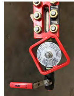
Conventional valves- such as Penberthy 330J / 320J can Seize with only trace amounts of H 2 S
